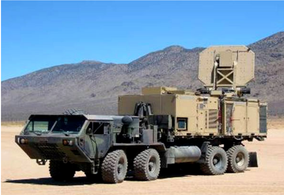
An operational version of the Active Denial System, a military counter-personnel directed energy weapon that is the equivalent of science fiction's heat ray. (Unlisted USAF personnel/Public domain/ Wikimedia Commons )
