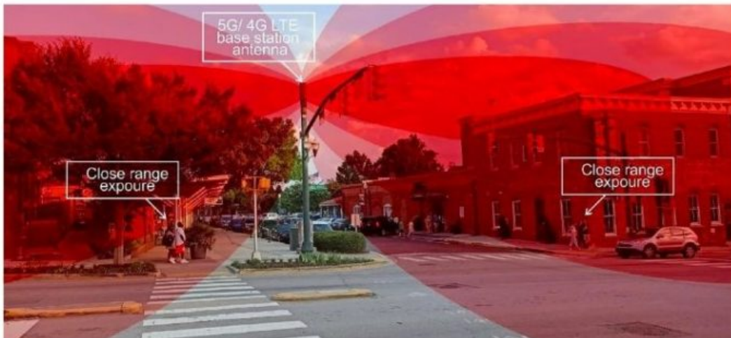
Figure 7. Gervais Street: Cell phone base station antenna placed close to street level and causing high exposure to pedestrians and nearby café visitors (exposure scenario illustration). The antenna appears camouflaged and seemingly part of a utility pole. The measurer only discovered the antenna due to the
