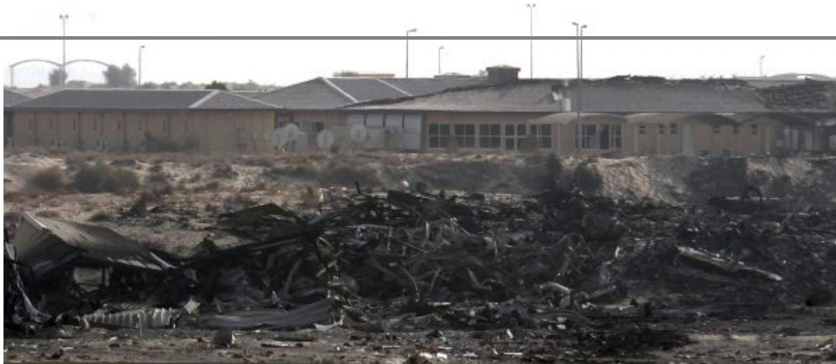
The remains of a UPS 747-400 Boeing cargo plane that went up in flames due to lithium batteries on Sept. 5, 2010. (AP Photo)
