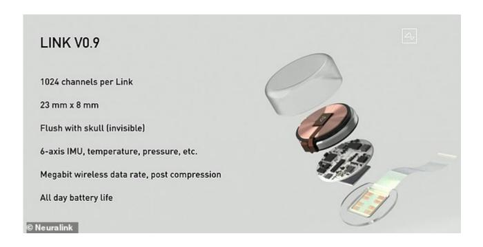
Neuralink's system is comprised of a computer chip attached to tiny flexible threads that are stitched into the brain by a 'sewing-machine-like' robot
