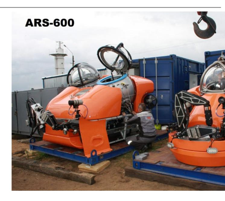
It should be noted that the ARS-600 submersible is designed for searching, examining and lifting various underwater objects from the seabed, sustaining life activity of crews in distressed submarines, as well as docking other rescue facilities with distressed submarines. The ARS-600 submersible has a double-hulled design and can be controlled from any of the hulls. Sonar systems are used for navigation and communication.
